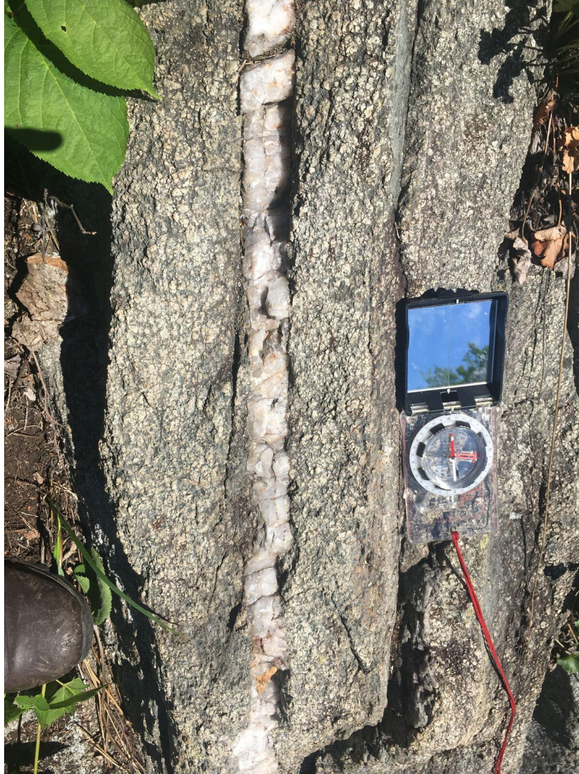
Figure 8: Granitic unit intruding the northwest quadrant of the property containing an undeformed quartz vein.
